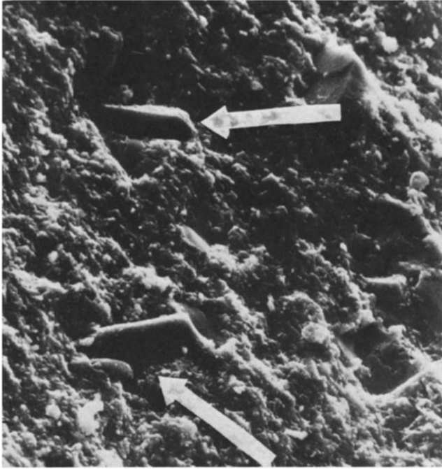
Fig. 2. SEM micrograph of a fracture face of a platelet composite showing intergranular crack propagation with respect to platelets.
